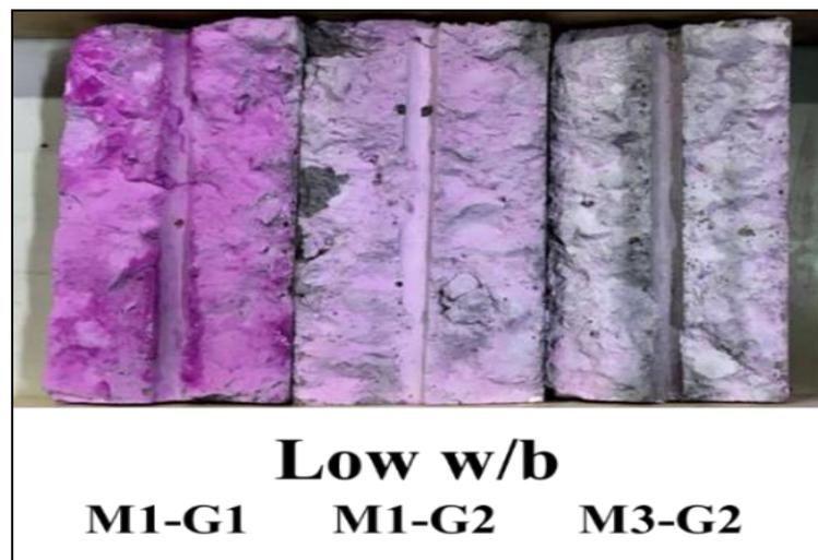
Figure 8 Results of water penetration into the bond area
