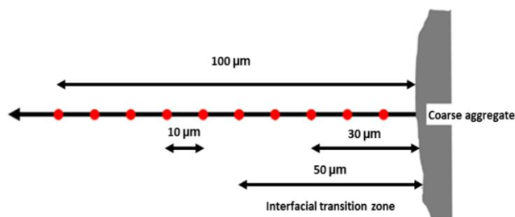
Figure 3 Measuring point of Vickers hardness
