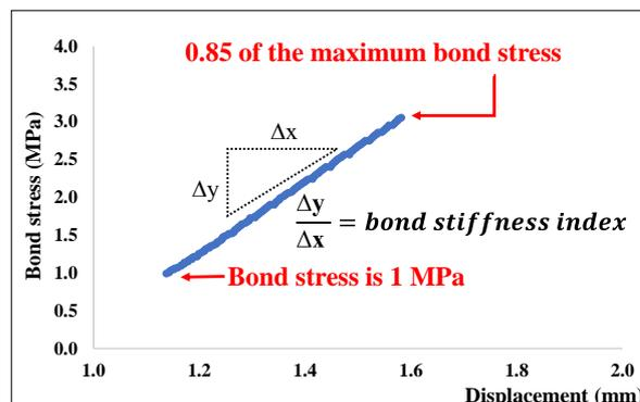
Figure 6 Test result of bonding pullout test
