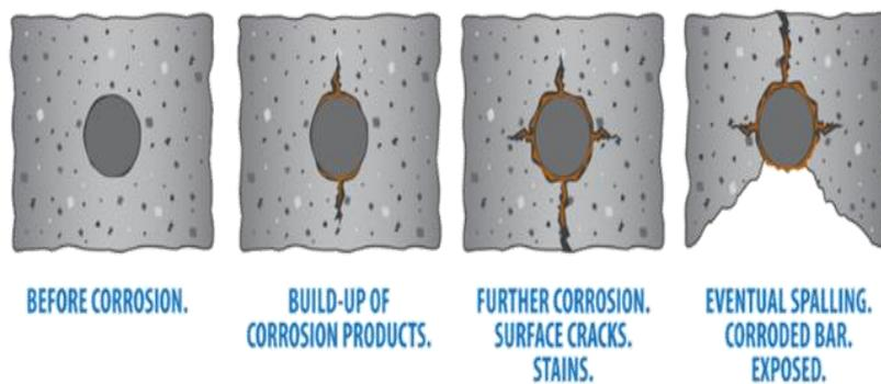
Figure 2 Process of steel corrosion in concrete
