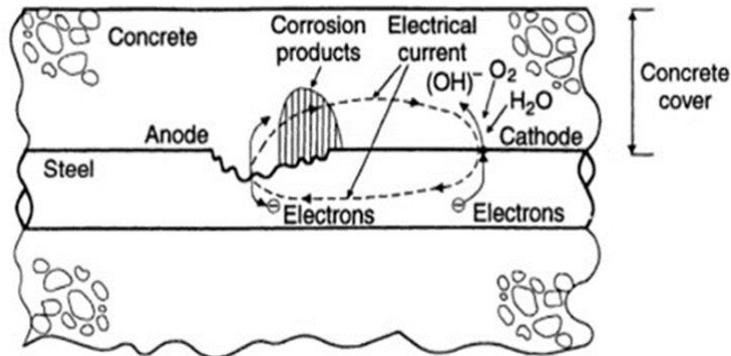
Figure 1 Electrochemical process of steel corrosion in concrete
