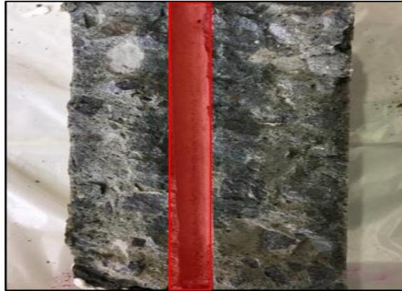
Figure 4 Focused area for water penetration test
