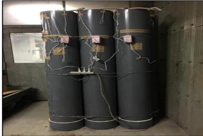
Figure 5 Cylindrical tanks for wet and dry cyclic test
